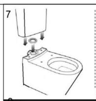
7. Place rubber seal into pan recess (DO NOT USE SEALANT). Place cistern screws into holes on the inside of cistern, making sure washers are located correctly. Gently lower cistern onto pan locating fixing screws into matching pan screw holes. Secure cistern to pan. Before tightened fully make sure cistern sits square and straight to
