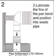
Pipe A(Standard):70-150mm Pipe B:100-190mm Pipe C:150-250mm
